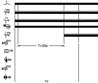
Continuous prepurge state with switching time of PA > 20s and pressure switch opening in running position.
