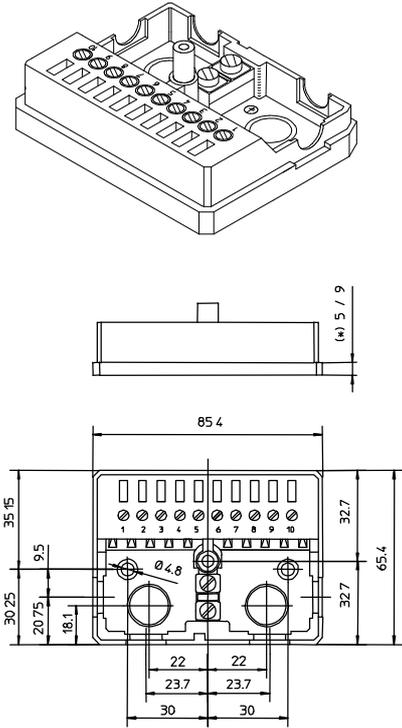
(\* The dimensions differ depending on the type of socket: 5 with socket D, 9 with socket E
